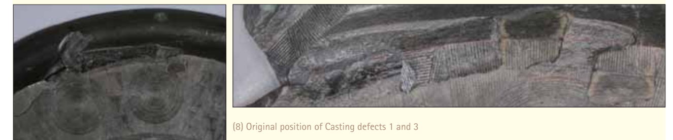
(7) Location of Casting defects 1, 2, 3
