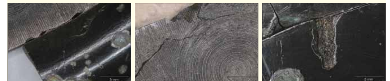
(4) Rat-tail defect and scab on the lower part of the outer section and rim
