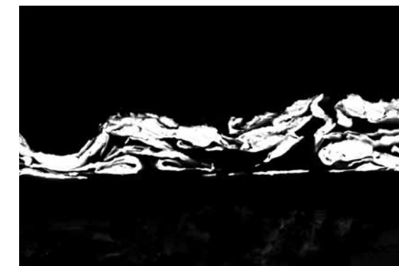
Fig. 52. Cross-section of the lacquer around the gilt designs 2 (SEM).
