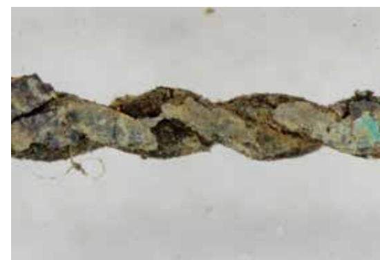
Fig. 45. Double-stranded wire.
