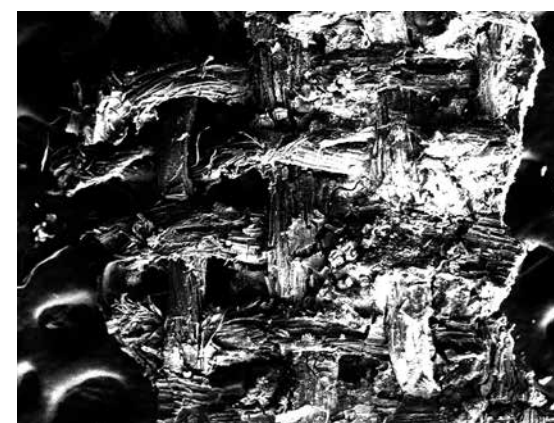
Fig. 35. Weaving of the fabric base (SEM of the backside of the lacquer layer).
